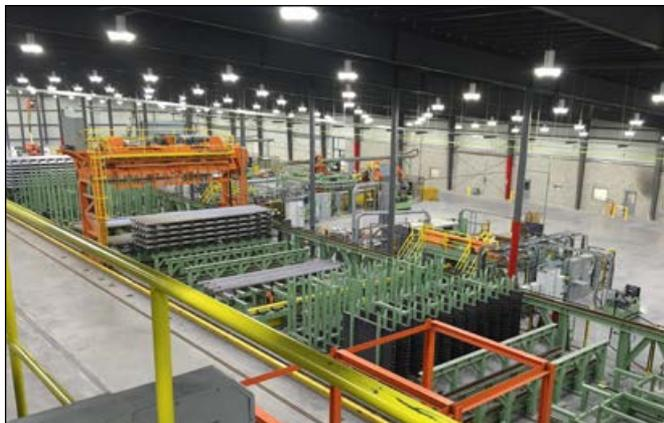
Figure 7. Overview of the billet handling system. The infeed conveyor at bottom right carries the billet to the load build table, where a bundle is formed for the homogenizing ovens. Two of the three sawing lines can be seen in the background.
