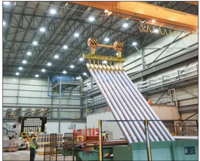
Figure 5. The new vertical casting system can cast billet up to 300 inches in length.
